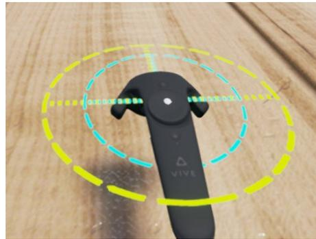
(b) Activation - the pad has been just pressed, *origin pose* is stored and represented with the green marker.
