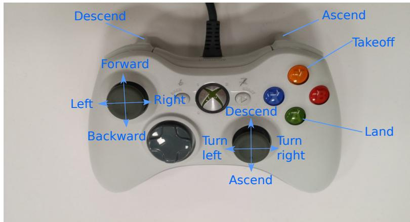
Figure 5.1: The traditional analog stick control scheme utilized in the user study.
